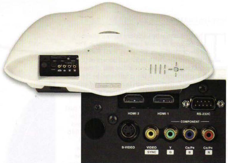
ABOVE: The video inputs could not be more straightforward – composite, component and S-video support older analogue sources while a choice of two HDMI sockets is available for digital video from modern DVD/HD DVD/Blu-ray players and set-top boxes
